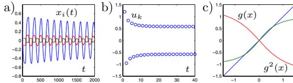
Fig. 2. The same system is considered as in Figure 1, except that the value of  $\mu_1$  has been changed to 0.09. The typical solutions of a) system (1) and b) system (4) now appear to be limit oscillations and periodic 2-cycles. c) In this case  $|g'(x_0)| = 1/0.9 > 1$  and  $g^2(x) = x$  has several solutions.
