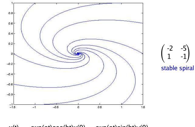
$\begin{aligned} x(t) &= \exp(at)\cos(bt)x(0) - \exp(at)\sin(bt)y(0) \\ y(t) &= \exp(at)\sin(bt)x(0) + \exp(at)\cos(bt)y(0) \end{aligned}$
