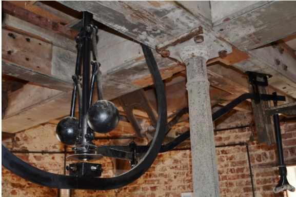
centrifugal governor at a restored windmill in moulton, lincolnshire, UK. design like this date to the 18 th century
