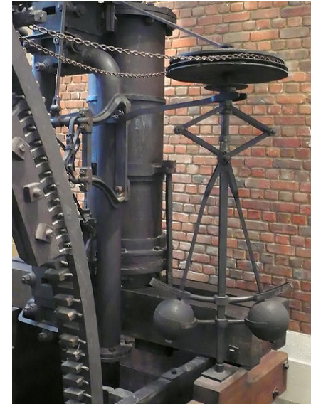
Boulton-Watt steam engine with a centrifugal governor
