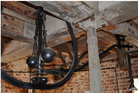
centrifugal governor at a restored windmill in moulton, lincolnshire, UK, dating from the 1820s
