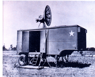
SCR-584 gun control radar
